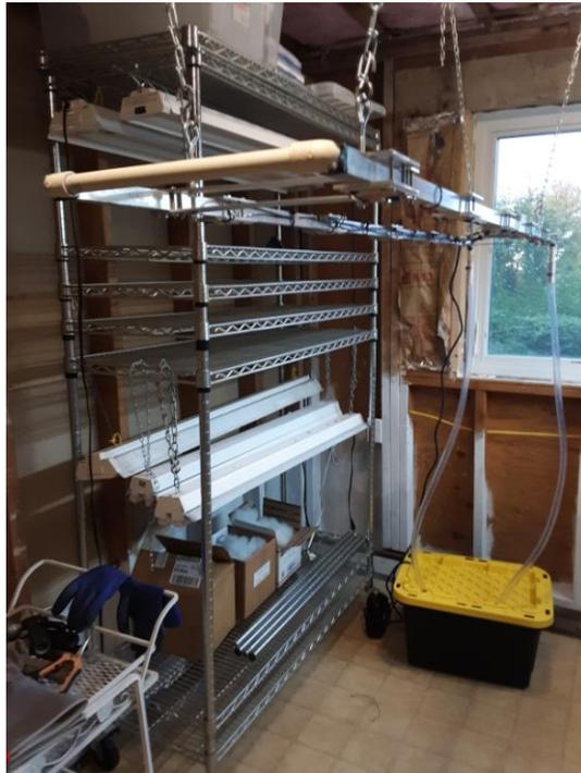
This unit was built for a friend and was designed to fit the space and plants in his growing area. It can be built in many configurations as a person wishes to have. It can be used indoors or outdoors in a greenhouse setting. This unit was about 500 watts and cost about \$150 to build.
