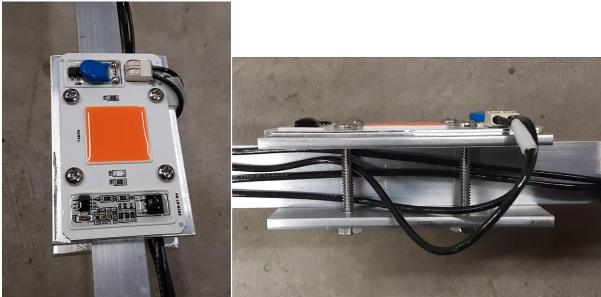
After mounting the LED s the way you want, then it's just a matter of connecting the wires to each. This is a nice design on these at it is simply pushing the wire into the white connector. All of these go to a waterproof box (gray) that has screw on terminal connectors in it.
