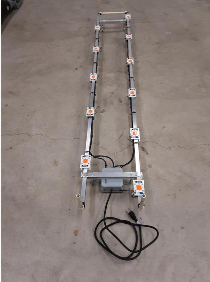
Let's start out with the finished product. This one has 11 lights on it. We will be using an LED light called a chip on board (COB). Each COB has its own built in circuit so that all is needed is to provide normal house current to make it work. All are mounted on square aluminum to provide cooling.
