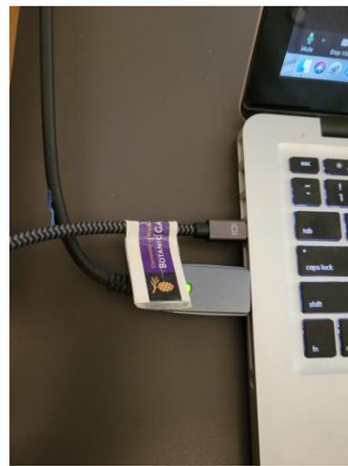
**HDMI video connector on top. USB audio on bottom with green light.**
